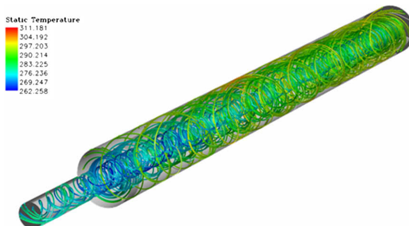
Fig. 18. Three-dimensional visualization of streamlines patterns with temperature map, obtained by LES with Smagorinsky closure model.
